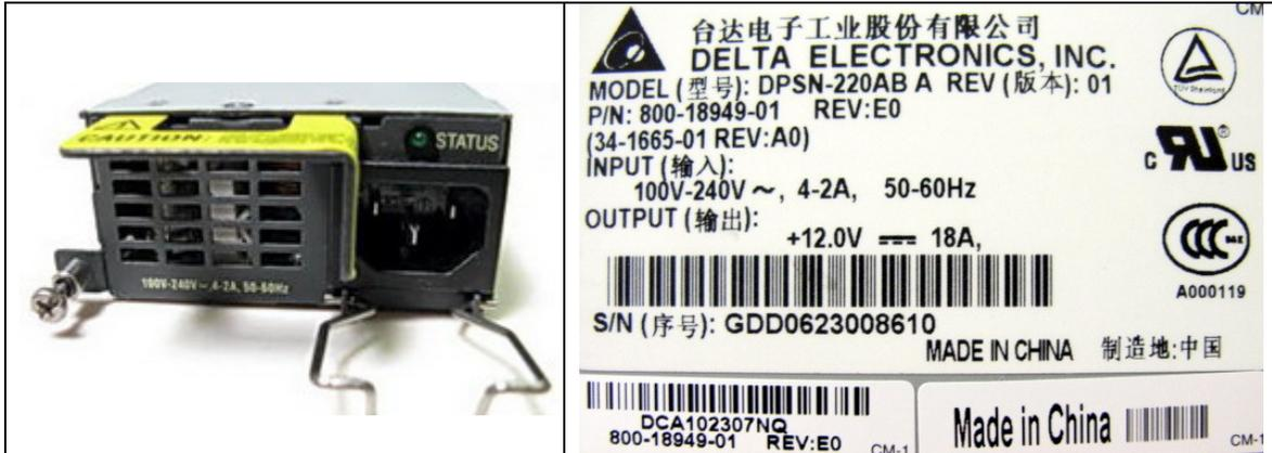
This is a universal AC input (100-240V) modular (plug in) 220W supply that outputs a nominal 12VDC at up to 18A. It has a standard IEC line cord connector (with plug retainer) and green status light (when operating). **There is no fan inside the unit, but forced air (from within the cabinet) to exhaust the supply is a good idea above 10A to control heat build-up.**
