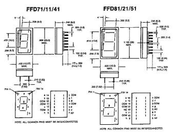
The IEE APOLLO readout consists of segmented tungsten filament characters with decimal point on a black ceramic base sealed in a glass tubular envelope. The displays provide ultra-wide viewing angle and superb readability. Extra long life is assured by rugged unitized construction. Brightness is fully adjustable from zero outout to a level easily viewed in direct sunlight by simply varying the voltage. Any desired filter color may be used.
