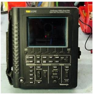
In my case, I started with a filthy dirty unit, covered in foam crumbles from the storage bag. It had both a dead battery, and dead wall-wart charger. In addition, the twist cap that holds the battery in place broke apart. I replaced the wall-wart with a nice stock 12VDC/1A linear unit, and that worked great. The battery was much more of a problem. In my unit, the original Tek pack had failed, and somebody had made a replacement using NiCad cells as shown below:
