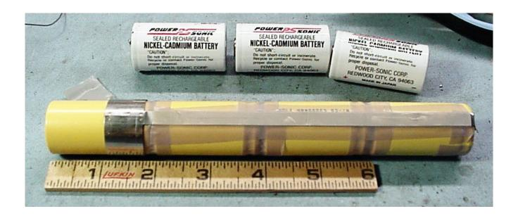
I removed the contact ring from the old pack, and attached the positive contact ring and runner to the + end of the pack (now at the RIGHT in the picture above) insulate under with teflon tape to prevent shorts when soldering, and secured it in place with tape, so that the contact was correctly positioned and secure. Its top end lines up close to the top of the first cell at the left (whose negative terminal forms the negative contact).
