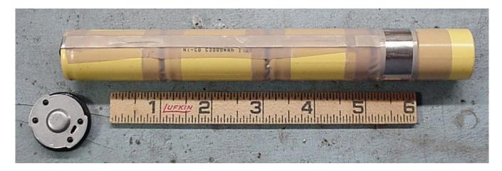
I then taped the edges of the contact carefully in place, so it would not catch on anything when inserted, and covered as little metal as possible. I also epoxied the battery cap back together, and heated it to be certain the epoxy would cure properly. I left that for 24 hours to set. Do not try any form of crazy glue, it won't work.
