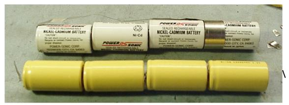
Note the strange metal band on the original cells, we will recycle that later as the positive (+) battery contact. I left it in place so I would know the correct position it needed.
