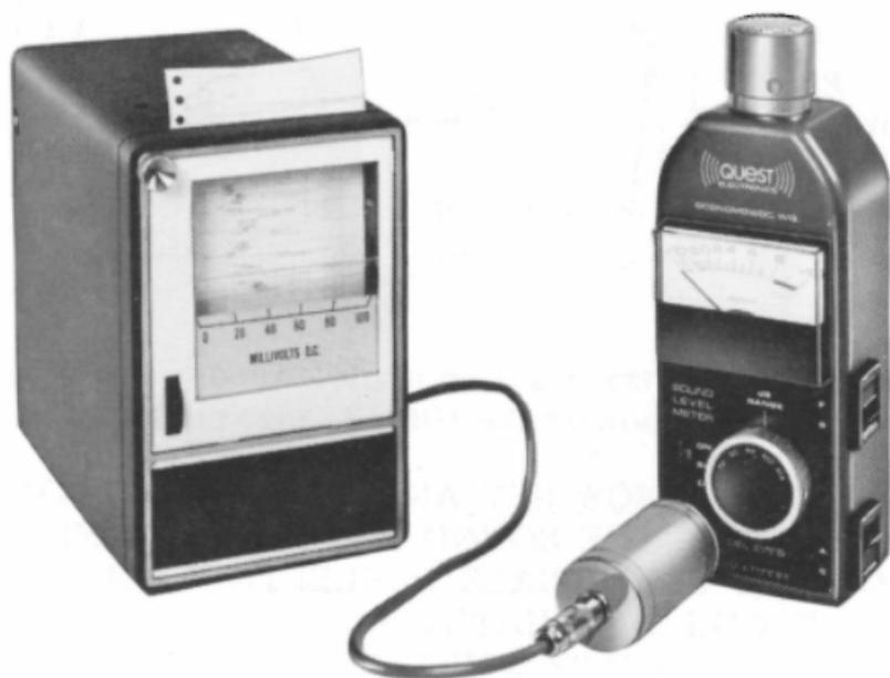
**211FS Meter Connected to DC Recorder
