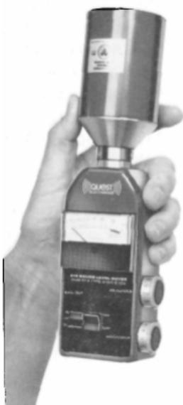
inside coupler resting flush on the inner rim. The 110 decibel output of the calibrator should produce a full scale +10 reading on the meter. If the Model 211AR or 211FSR Sound Level Meters are used with a microphone extension cable, then calibration is performed with the microphone mounted on the extension cable. Note the correction in calibrator output due to altitude effects on page 21.
